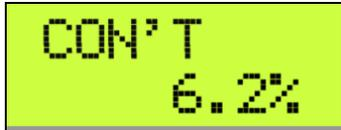
**2.4.2** While pressing and holding the Quick Selection Button
